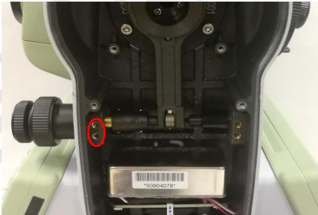
Figure 2-15 fixing screws
