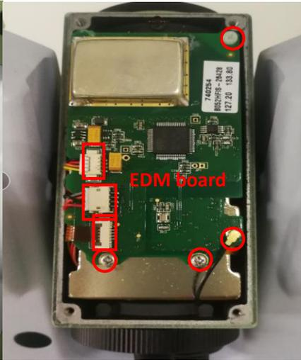
Figure 2-5 EDM board,cables and screws
