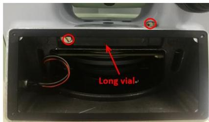
Figure 2-13 long vial and screws
