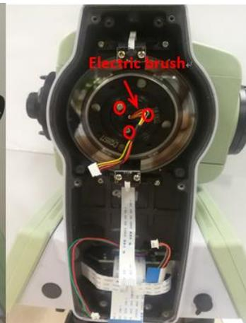
Figure 2-10 electric brush and fixing screws
