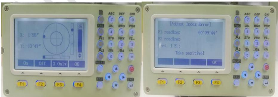
4) Face 2: do the same thing as done on Face 1, and finally press **【Ok】** and restart the instrument to save the parameter.
