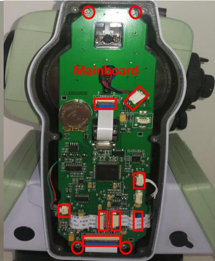
Figure 2-8 main board , cables and screws
