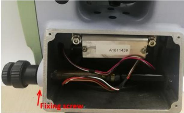
Figure 2-14 fixing screws
