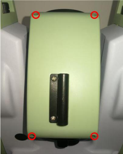
Figure 2-4 telescope cover screws
