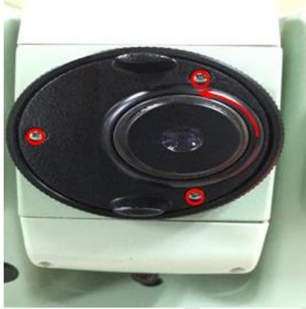
Figure 2-16 eyepiece, protective cover, screws
