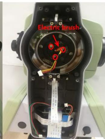
Figure 2-10 electric brush and fixing screws
