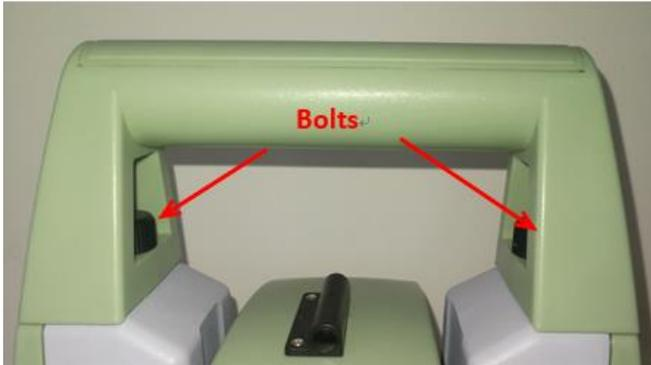
1. Unscrew the two bolts with hand then take out the handle unit.
