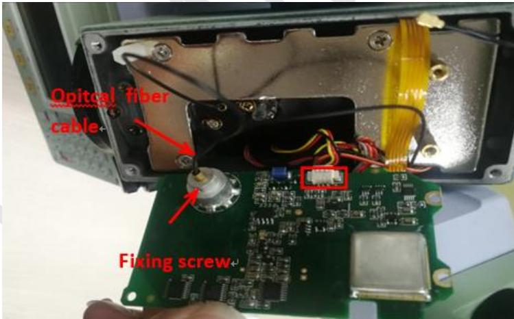
Figure 2-6 optical fiber cable
