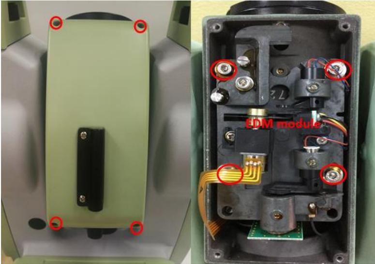
Figure 2-11 telescope cover screws
