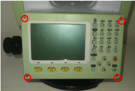
Figure 2-2 display screws
